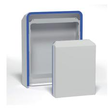
Powder-coated steel cover RAL 7035, to be applied to exhaust filters and filter fans to protect the internal components of the electrical panel from water jets and the ingress of solid objects, in order to elevate the protection rating to IP56. Also available in stainless steel (AISI 304) and with FDA-compliant gasket for applications with high hygienic standards in the Food & Beverage sector and for outdoors.
