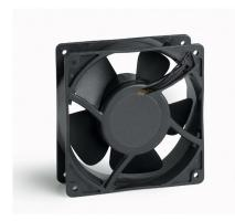
An EC fan (stand for Electronically Commutated) is a brushless, direct current, motor. This runs on a DC voltage, but with a single phase AC supply. Thanks an electronic PCB board included in the stator, single phase AC voltage is transformed into a direct voltage by an AC/DC converter. EC motors assure energy efficiency, quiet operation and high performances.
